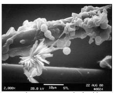
Scanning electron micrograph of mold growth encircling a fiberglass fiber May Indoor Air Investigations LLC
