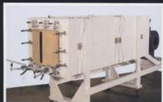
An airflow test chamber was built to ANSI/ASHRAE 210 specifications
