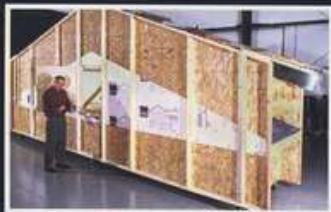
An attic simulator was built to test ridge vents
